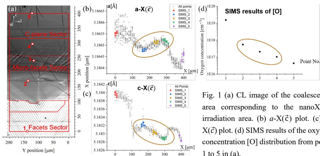
Fig. 1 (a) CL image of the coalescence area corresponding to the nanoXRD irradiation area. (b)  $a$ - $X(\vec{c})$  plot. (c)  $c$ - $X(\vec{c})$  plot. (d) SIMS results of the oxygen concentration [O] distribution from point 1 to 5 in (a).
