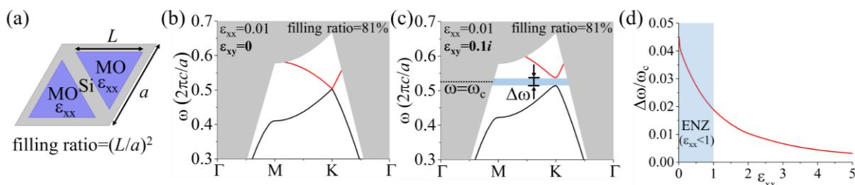
**Fig.1** (a) Schematic of a unit cell of the investigated PhC. (b,c) Band structures of the non-magnetized (b) and the magnetized (c) ENZ-MO PhCs, respectively. (d) Variation of  $\Delta\omega/\omega_c$  with respect to  $\epsilon_{xx}$ . All calculation results in (b-d) were obtained by using the commercial software package COMSOL Multiphysics.
