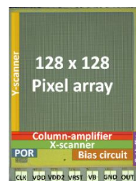
Fig. 1 Photograph and specifications of the fabricated CMOS image sensor.
