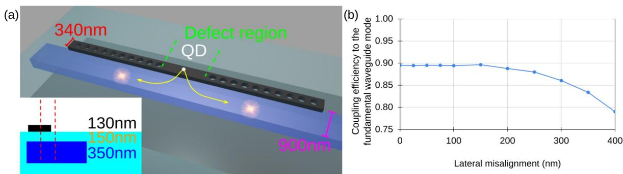
**Fig. 1** (a) Schematic of the defect-based nanobeam cavity integrated on the SiN waveguide. The inset shows a vertical cross-section of the structure, showing the thicknesses of the nanobeam cavity, vertical separation, and the waveguide. The lateral distance between the red dash lines is the lateral misalignment. (b) Coupling efficiency into the fundamental guided mode as a function of lateral misalignment.
