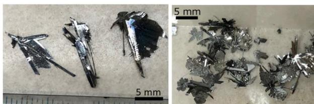
Fig. 3 Optical images of the  $\beta$ - $\text{MoTe}_2$  crystal grown by CVT using 50 mg Cl (left) and 50 mg I (right) as a transport agent.
