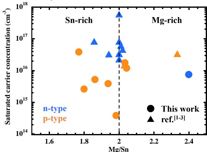
Fig.2 Saturated carrier density and conduction type.
