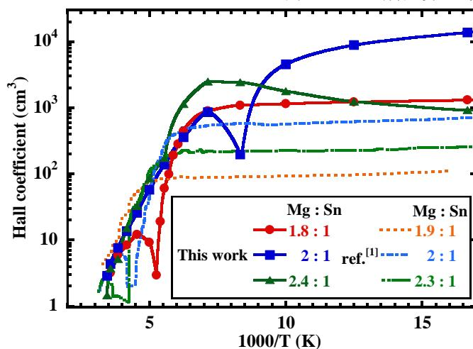
Fig.1 Temperature dependence of Hall coefficient.
