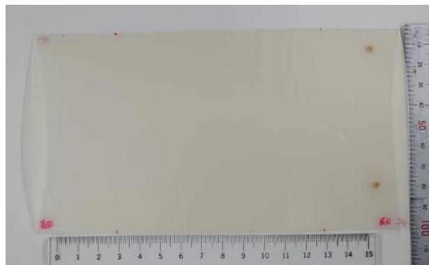
Fig. 1. Image of the multiple AlN and Al<sub>2</sub>O<sub>3</sub> films
