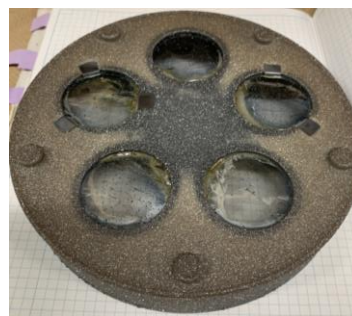
Fig.1 Photograph of susceptor after growth of GaN on ScAlMgO 4 . GaN substrates were separated from ScAlMgO 4 substrates.
