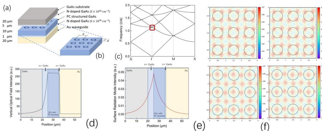
Fig 1. Simulated SEQCL's structure sketch and its photonic crystal structured QCL layer are shown in (a) and (b). (d) and (e) are guided mode vertical optical profile and surface radiation intensity curve with fundamental modes' pattern are shown in (f).
