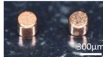
Fig. 2 A photograph of copper pillars fixed on Rivalpha.
