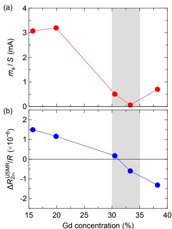
Figure. (a) The Gd concentration dependence of the saturation magnetic moment per area and (b) the normalized USMR at a current density of  $0.3 \times 10^{11}$  A/m<sup>2</sup>.
