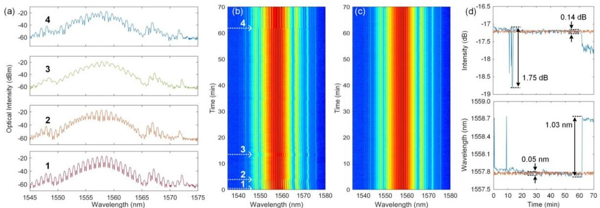
Fig. 2 (a) Four transition states in (b) long-term continuous operation without temperature feedback; (c) Results with temperature feedback; (d) Variation of the central wavelength and its power density.
