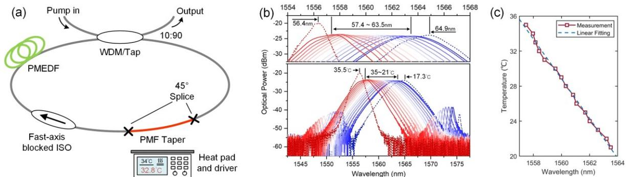
Fig. 1 (a) The schematic diagram of the tunable laser; (b) Spectra and (c) linear relationship of temperature-controlled wavelength tuning.
