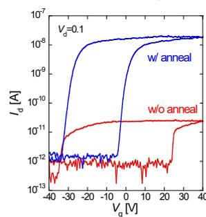
Fig.2  $I_d$ - $V_g$  characteristics in 300-nm-thick SiO<sub>2</sub>/MoS<sub>2</sub> n-FET w/ and w/o annealing.
