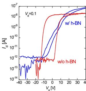
Fig.4  $I_d$ - $V_g$  characteristics in 300-nm-thick SiO<sub>2</sub>/MoS<sub>2</sub> n-FET w/ and w/o insertion of h-BN interfacial layer.
