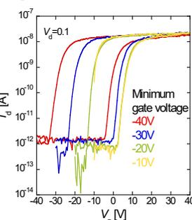
Fig.3  $I_d$ - $V_g$  characteristics in 300-nm-thick SiO<sub>2</sub>/MoS<sub>2</sub> n-FET with different minimum gate voltage.
