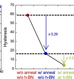
Fig.5 Hysteresis of MoS<sub>2</sub> n-FET w/o anneal and w/o h-BN, w/ anneal and w/o h-BN, w/ anneal and w/ h-BN.
