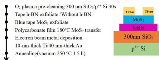
Fig.1 Process flow and device structure of 300-nm-thick SiO<sub>2</sub>/h-BN/MoS<sub>2</sub> n-FET
