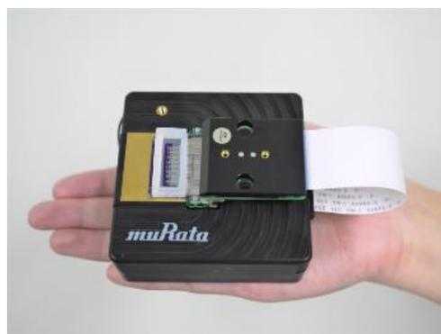
Fig.1 Prototype of Graphene FET
