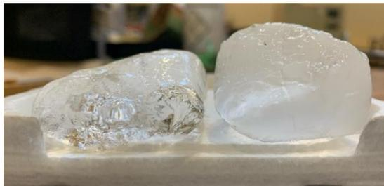
Figure 1. Ice with (Left) and without (Right) electron beam shielding, Ice is after 3 shots.
