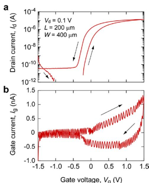
**Figure** | (a) Typical transfer characteristic curve and (b) gate current of the resultant ITZO-FeTFT. Anticlockwise hysteresis with memory window of 0.2 V is clearly seen in (a).
