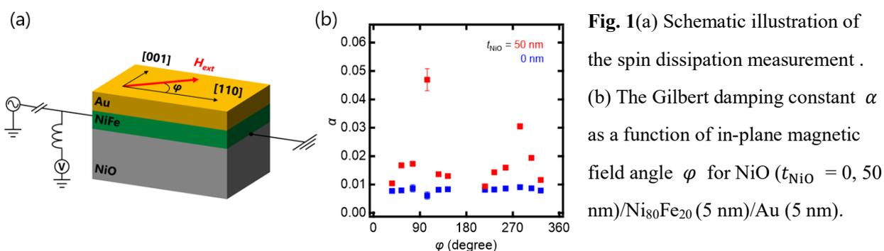
**Fig. 1** (a) Schematic illustration of the spin dissipation measurement. (b) The Gilbert damping constant  $\alpha$  as a function of in-plane magnetic field angle  $\varphi$  for NiO ( $t_{\text{NiO}} = 0, 50 \text{ nm}$ )/Ni<sub>80</sub>Fe<sub>20</sub> (5 nm)/Au (5 nm).
