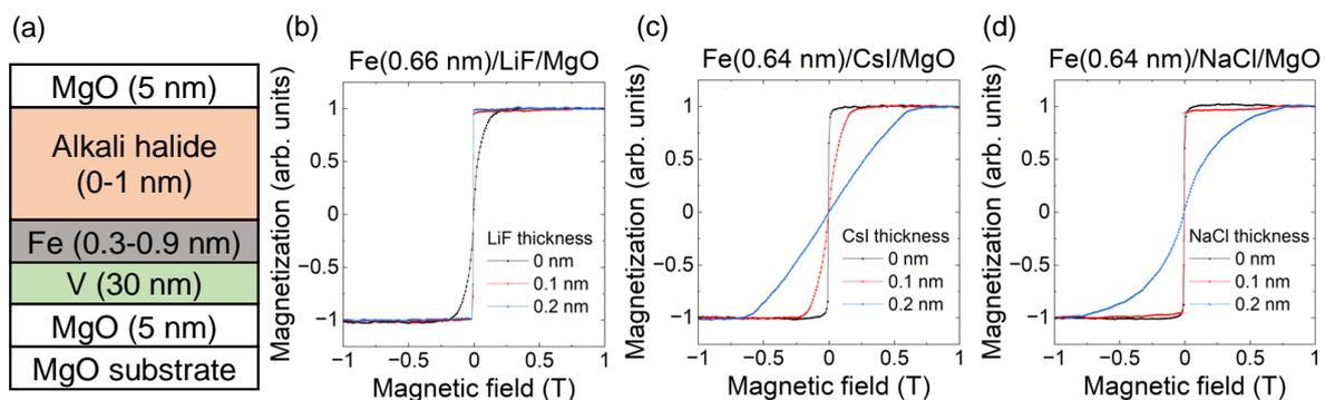
Fig. 1. (a) Schematic sample structure. Normalized out-of-plane magnetization curves for (b) LiF-, (c) CsI-, and (d) NaCl-inserted samples.
