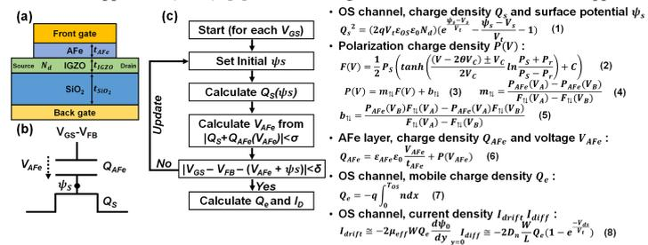
**Fig. 1** Simulation framework of AFefFETs with OS channel. (a-b) Schematic illustration of simulated device structure, (c) modeling and simulation flow chart, and equations.
