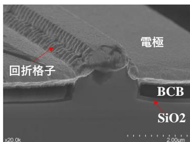
Fig.1 SEM image of fabricated QD-DFB-LD.
