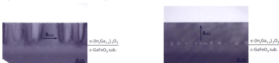
Fig. 2 Contrast experiment for the defects in the  $\kappa$ -(In<sub>x</sub>Ga<sub>1-x</sub>)<sub>2</sub>O<sub>3</sub> film under  $g=020$  and  $g=002$ .
