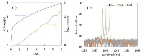
Fig. 2. (a) Measured V/I & L/I, (b) lasing spectra
