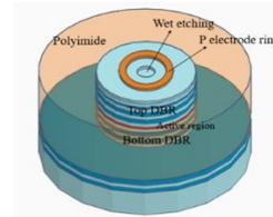
Fig. 1. Schematic structure of 1060nm intra-cavity metal aperture VCSEL.
