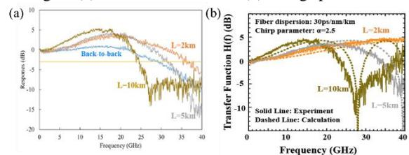
Fig. 3. (a) Small signal modulation response through different lengths of SMF, (b) Transfer function of SMF transmission with different fiber lengths in comparison with the calculation
