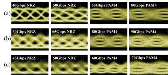
Fig. 4. Eye diagrams with different bit rates through (a) back-to-back, (b) 2km SMF, and (c) 5km SMF.
