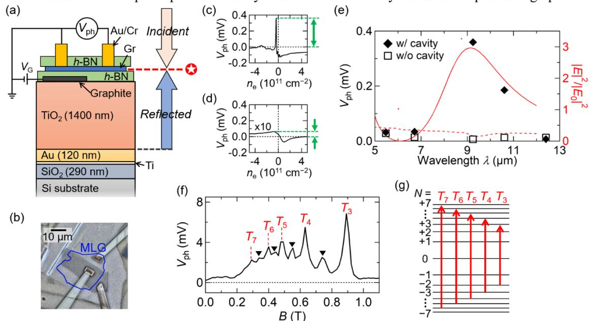
**Fig. 1:** (a) Device structure. (b) Optical micrograph. (c,d)  $V_{ph}$  data from the device (c) w/ cavity and (d) w/o cavity. (e)  $V_{ph}$  vs  $\lambda$ . (f)  $V_{ph}$  vs  $B$ . (g) CR transitions in monolayer Gr.
