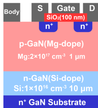
Fig.1 Schematic illustration of GaN-MOSFET.
