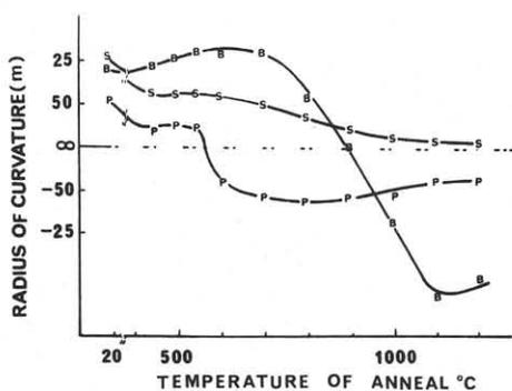
Fig. 1. The effect of annealing temperature on radius of curvature developed by changes of lattice location. B, P, and S show the experimental results from the wafers on which B, P, and Si atoms are implanted, respectively.
