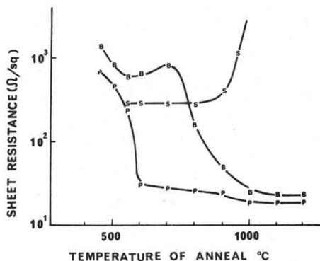
Fig. 2. Isochronal annealing of ion-implanted layers at various temperatures. Each annealing lasted 10 min. Signs B, P, and S are similar to those in Fig. 1.
