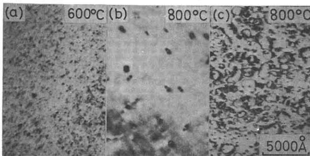
**Fig. 2.** Micrographs of defects in 20°C Si<sup>+</sup> ion implanted GaAs annealed at various temperatures for 1 hour (Impl:  $1 \times 10^{13}/\text{cm}^2$  (a) and (b),  $1 \times 10^{15}/\text{cm}^2$  (c)).
