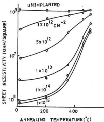
**Fig. 1.** Changes in the layer resistivity by 1 hour isochronal annealing (20°C Si<sup>+</sup>impl.).
