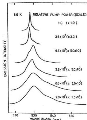
Fig.2 Spectral change with pump power
