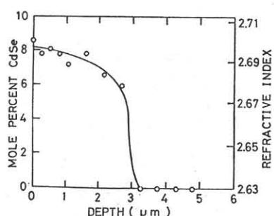
Fig.1 Distribution of CdSe in the mixed crystal layer
