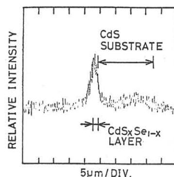
Fig.3 Microphotometer trace of the near field pattern
