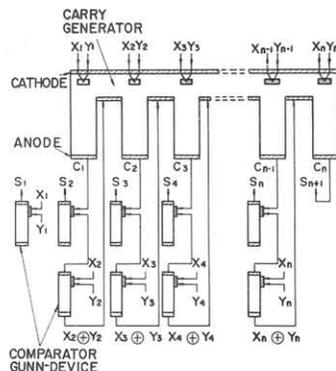
Fig.1 An N-bit full adder composed of a comb-shaped carry generator and exclusive-OR (comparator) using Gunn effect
