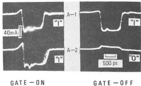
Fig.3 Current waveforms for each stage in 2-bit carry generator. Upper two traces are those for the first stage when the ohmic gate is 'ON' and 'OFF'. Lower two traces are for the second one.
