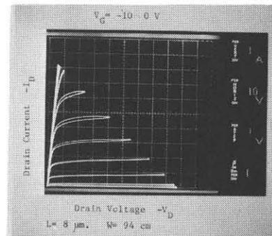
Fig.5 Typical static characteristic of the fabricated device.
