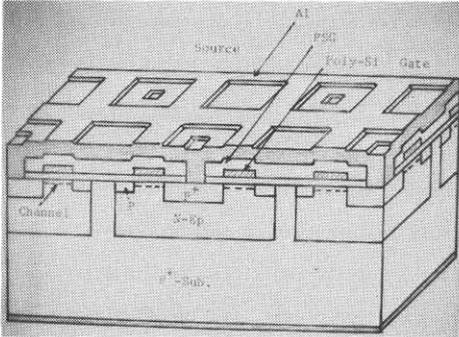
Fig.2 Schematic cross section of the high power MOSFET.
