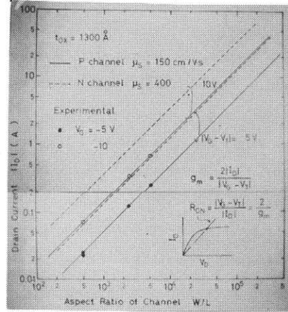
Fig.1 Drain current as a function of channel aspect ratio in the high voltage MOSFET.
