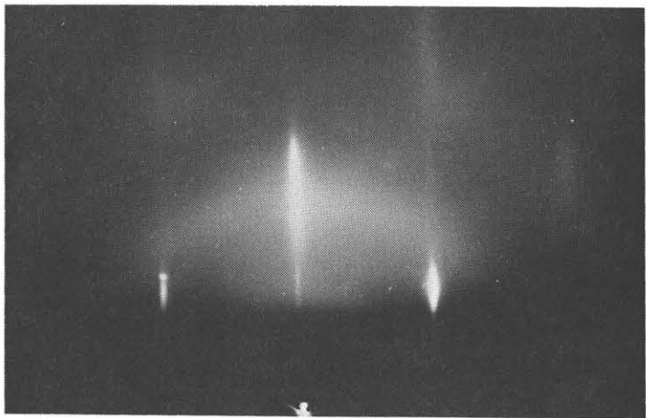
Fig.1 RHEED pattern of ZnSe MBE layer. 50 keV [100] azimuth.
