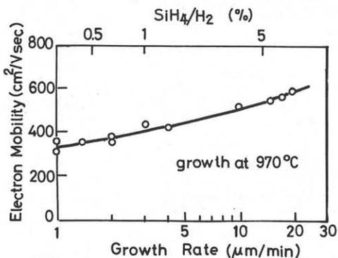
Fig.1 Electron mobility as a function of silicon growth rate and of silane content in hydrogen.
