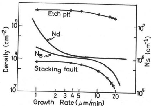
Fig.3 Calculated Nd and Ns, observed dislocation etch pit and stacking fault density versus growth rate.
