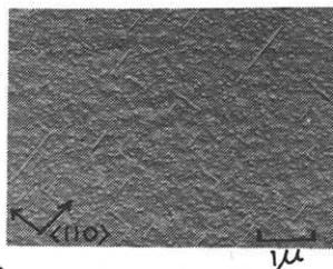
Fig.4 Etch pit and stacking fault on the film surface.
