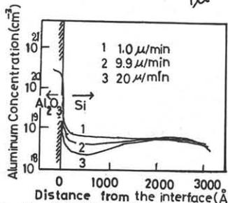
Fig.5 IMA profile of aluminum in the film.
