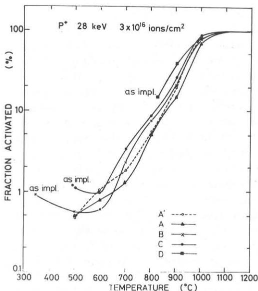
Fig. 1. Annealing characteristics of P<sup>+</sup> implanted Si as a function of dose rate.
