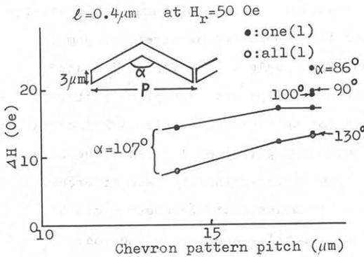
Fig.2. Bubble domain quasi-static stretch propagation margin dependences on the chevron pitch and the apex angle.
