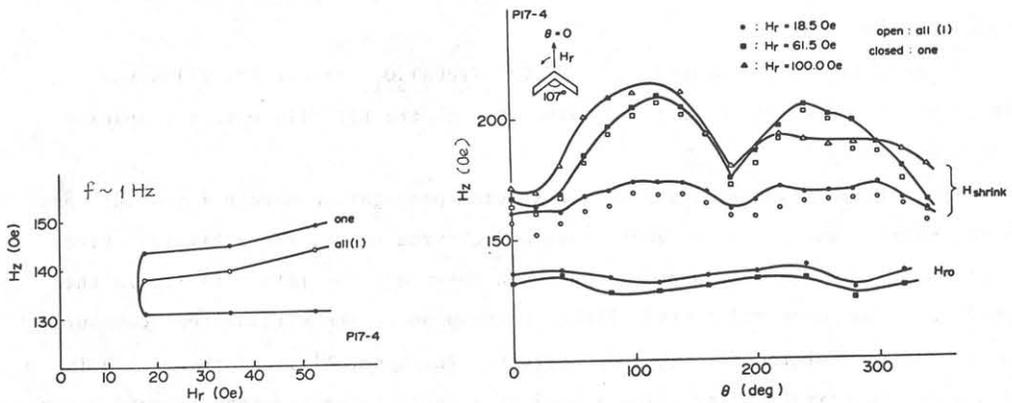
Fig.1(a). Bubble domain quasi-static stretch propagation margin on the  $17\mu\text{m}$  pitch chevron stretcher.
