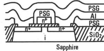
Fig.1 Cross section of the MOSFET.
