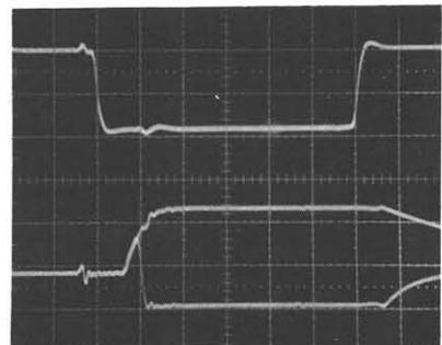
Fig.6 Oscillograph of SOS memory access time from chip enable;  $V_{CC} = 5$  V. (Horz. : 50 ns/div., Vert. : 2 V/div.).
