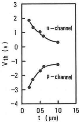
Fig.2 Threshold voltage of SOS-MOSFET's on the intrinsic film as a function of the silicon film thickness  $t$ ; the gates are doped n-type.
