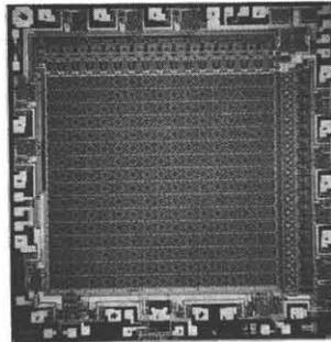
Fig.3 Photomicrograph of the synchronous static CMOS/SOS RAM.
