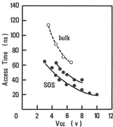
Fig.5 Access times of the fabricated SOS and bulk-silicon RAM's.
