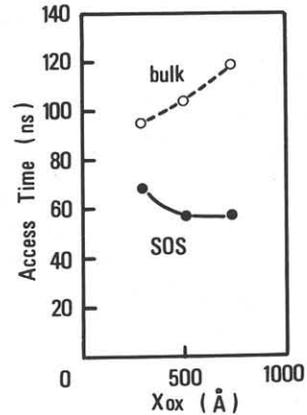
Fig.4 Simulated access times of the SOS and bulk-silicon RAM's as a function of the gate oxide thickness  $X_{ox}$ .  $V_{CC} = 4.4$  V.
