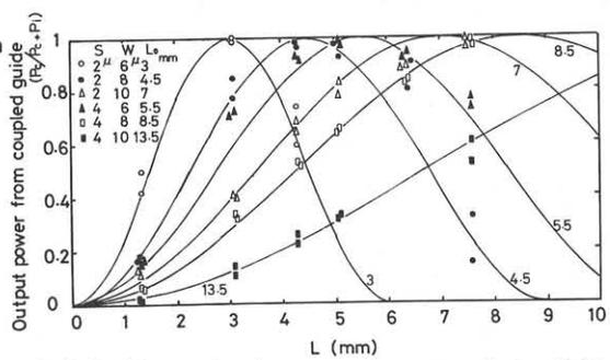
Fig.2 Relative output power from coupled guide of directional coupler.
