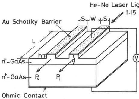
Fig.1 EDC switch with Au Schottky barriers
