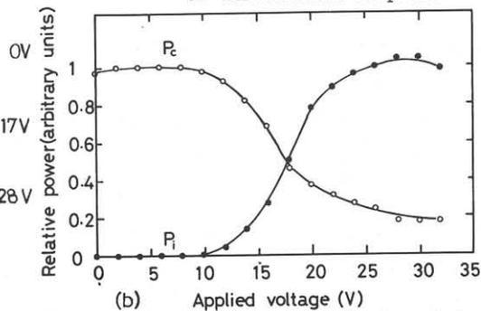
Fig.4(b) Relative power in the input and coupled channels as a function of an applied bias ( $S=4 \mu\text{m}$ ,  $W=8 \mu\text{m}$ ,  $d=4 \mu\text{m}$ ,  $h=1 \mu\text{m}$ )
