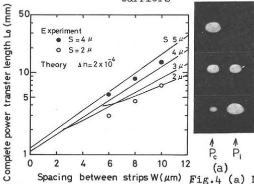
Fig.3 Complete power transfer length of directional coupler
