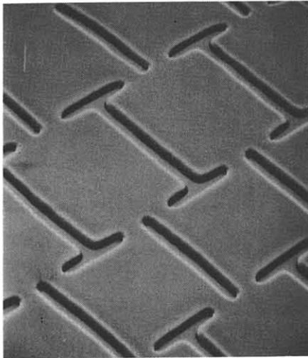
Fig. 2 Scanning electron micrograph of  $0.5 \mu\text{m}$  linewidth test patterns exposed in a resist film.
