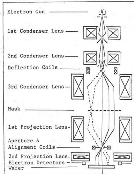
Fig. 1 Schematic of 1:4 demagnifying electron projection system.
