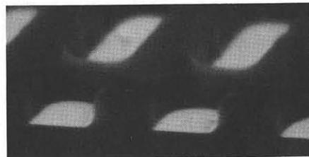
Fig. 3 Scanning electron micrograph of cross section of a  $0.5 \mu\text{m}$  linewidth grating pattern exposed in a resist film.
