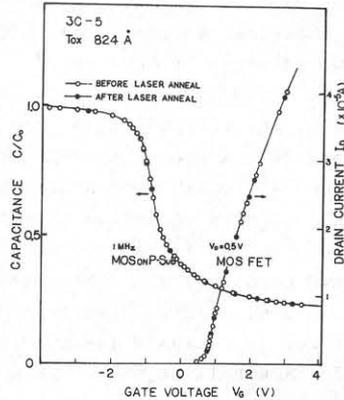
Fig. 6  $C-V$  and  $V-I$  characteristics of NMOS devices before (○) and after (●) laser anneal at a stressed condition.
