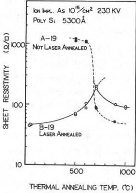
Fig. 1 Sheet resistivity of laser annealed and unannealed poly-Si as a function of subsequent thermal annealing temperature. As-ion dose is  $1 \times 10^{16} \text{ cm}^{-2}$ .
