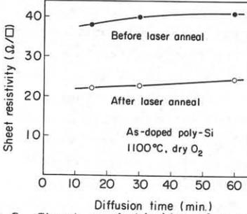
Fig. 3 Sheet resistivity of a poly-Si film, As diffused at  $1000^\circ\text{C}$ , as a function of diffusion time. Before (●) and after (○) laser anneal.
