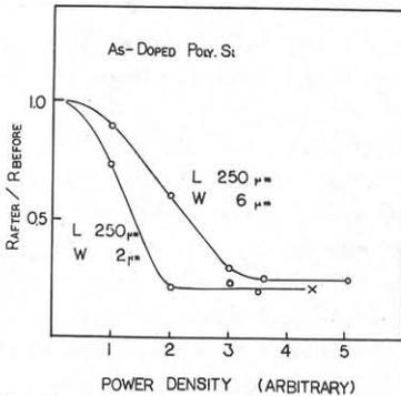
Fig. 5 Sheet resistivity change of patterned poly-Si lines,  $2\mu\text{m}$  and  $6\mu\text{m}$  width, by laser annealing.
