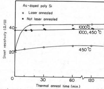
Fig. 4 Sheet resistivity of laser annealed and unannealed poly-Si as a function of subsequent annealing time, at  $450^\circ\text{C}$  and  $1000^\circ\text{C}$ .
