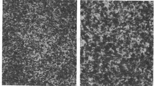
Fig. 2 Transmission electron micrographs of As-ion implanted, and subsequently laser annealed poly-Si. (a) before and (b) after subsequent thermal anneal at  $1000^\circ\text{C}$ .
