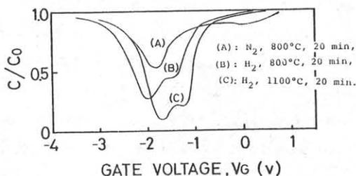
Fig.2 Low frequency C-V curves.
