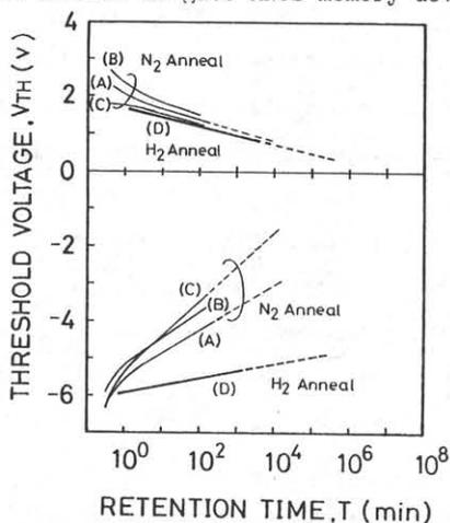
Fig.1 Retention characteristics of n-ch. Si-gate MNOST's.
