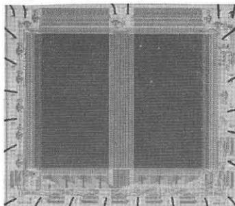
Fig.3 Microphotograph of the 16K EEPROM chip: size is 4x4.5 mm<sup>2</sup>.
