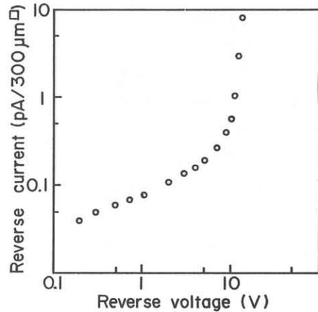
Fig.5 Reverse I-V characteristics of pn junction.
