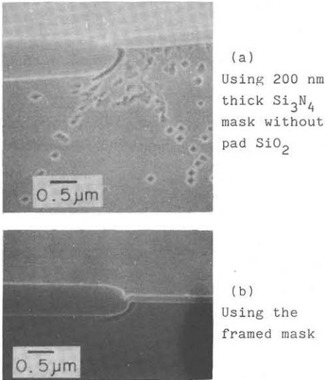
Fig.4 SEM cross sectional view of a silicon wafer etched with Wright etchant after selective oxidation.
