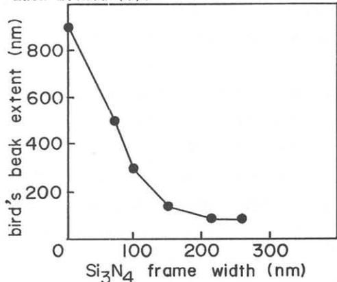
Fig.3 Bird's beak extent dependence on  $\text{Si}_3\text{N}_4$  frame width.
