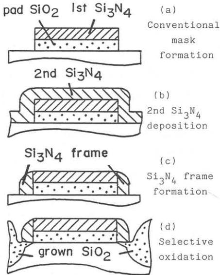
Fig.1 Selective oxidation process steps using the framed mask method.
