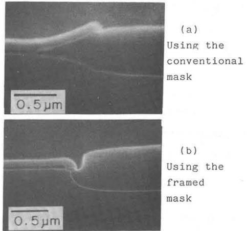
Fig.2 Oxide structures using conventional mask method (a) and framed mask method (b).
