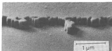
Fig. 4. SEM photograph of replicated PMMA pattern of Au mask. The sample is tilted to see the side wall of the pattern.
