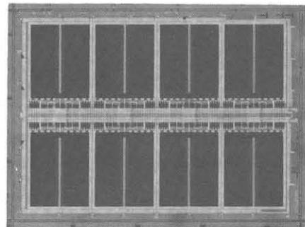
Fig. 3 Microphotograph of 512 kbit ROM chip
