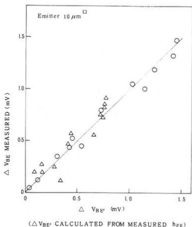
Fig.1. The relation of the  $V_{BE}$  values between measured and calculated from measured  $h_{FE}$  difference.
