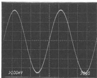
Fig.4. Reconstruction of a 10 kHz sinewave sampled at 40 MHz to 8 bit accuracy.
