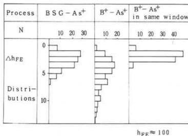
Fig.2. Typical distribution of the  $h_{FE}$  for various processes.
