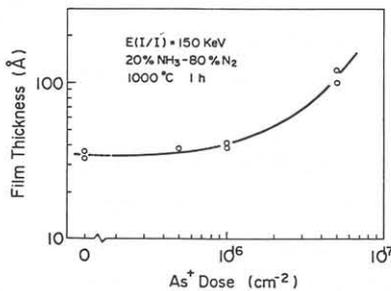
Fig.2 Dependence of the thermally grown silicon nitride film on As<sup>+</sup>dose.
