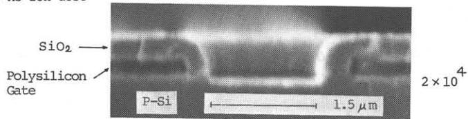
Fig.5 Cross sectional photograph of self-aligned contact.
