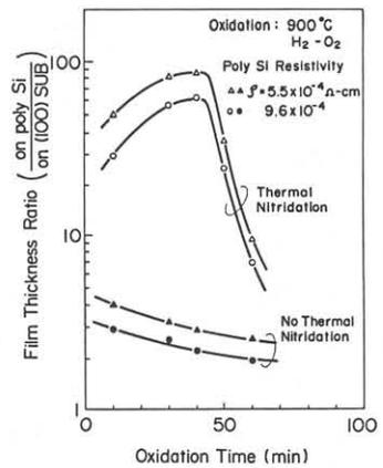
Fig.4 Film thickness ratio as a function of oxidation time.
