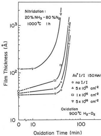
Fig.3 Oxidation-barrier effect of silicon nitride film as a parameter of As<sup>+</sup>ion dose
