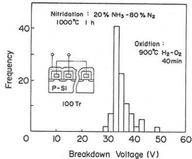
Fig.6 Breakdown voltage distribution of the oxide grown around the 100 SAC transistor polysilicon gates.
