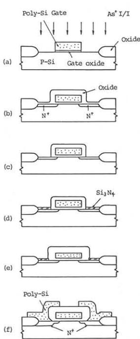
Fig.1 Schematic illustration of the self-aligned contact process.
