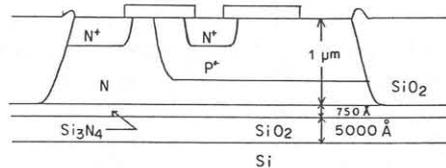
Fig.4 Cross sectional view of Bip-Tr. in SOI.
