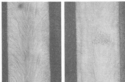
Fig.2 Optical micrographs of etched surfaces (a) recrystallized polysilicon on oxide at 10 W. (b) recrystallized polysilicon on nitride at 12.5 W
