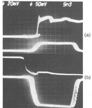
Fig.4(a) Response for the rise and (b) the fall. Trace of the light output (upper trace) and trigger current (lower trace).
