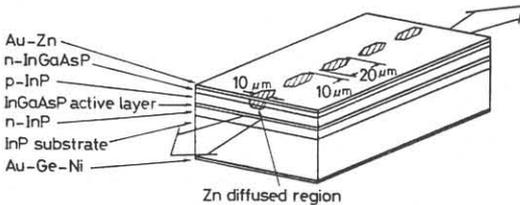
Fig.1 Structure of device. Injection regions are shaded.
