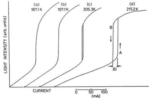
Fig.2 Typical observed I-L curves for CW operation. At 215.2K, a remarkable hysteresis loop is seen (curve d).  $\Delta I$  decreased with decreasing temperature, making direct bistability observation somewhat difficult (curve b, differential gain). At still lower temperature, the normal I-L curve is observed (curve a).
