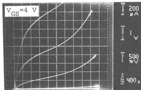
Fig.4 I<sub>D</sub> - V<sub>DS</sub> characteristics for parasitic transistor with L = 1.6 μm of isolation region ( V<sub>BB</sub> = -3 V )
