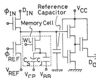
Fig.2 Equivalent circuit diagram of test device for C<sub>S</sub> measurement
