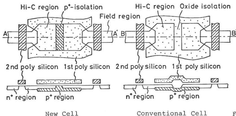
Fig.1 Memory cell structure of new cell and conventional one
