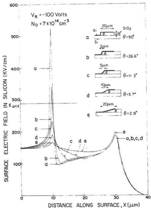
Fig. 1 Electric field distribution along the silicon surface of the Schottky diode shown in the inset for several taper angles.
