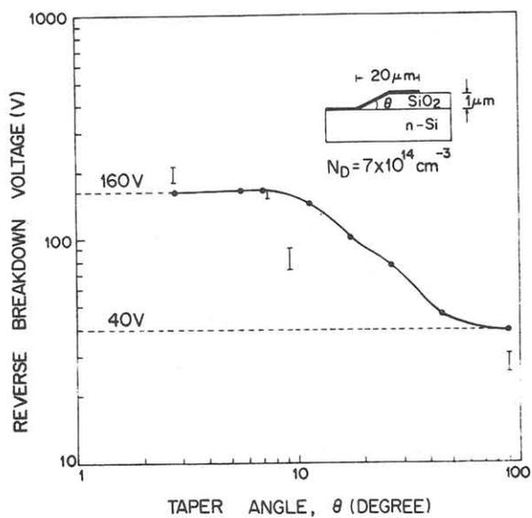
Fig. 2 Relationship between reverse breakdown voltage and taper angle for Al-n Si Schottky diode by numerical analysis. Experimental values are represented by the error bar, "I".
