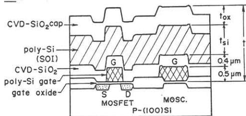
Fig.1: Cross sectional view of a sample used in e-beam annealing.  $t_{si}$ ; poly-Si(SOI) thickness,  $t_{ox}$ ; SiO<sub>2</sub> cap thickness,  $t$ ; thickness from surface to gate oxide.
