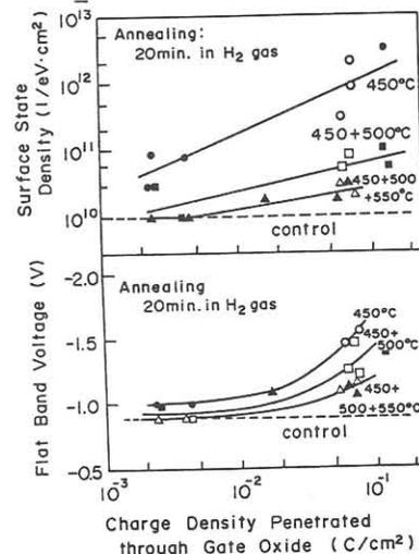
Fig.3: Surface state density and flat band voltage vs. charge density penetrated through gate oxide. Open symbol; SOI was melted, closed symbol; SOI not melted.
