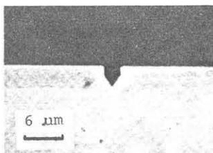
Fig. 1 The cross-sectional view of the groove etched by HCl.
