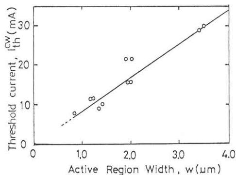
Fig. 3 The dependence of the threshold current  $I_{th}^{CW}$  at room temperature on the active region width  $w$ .
