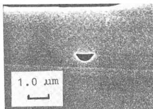
Fig. 2 The s.e.m. photograph of narrow active region.
