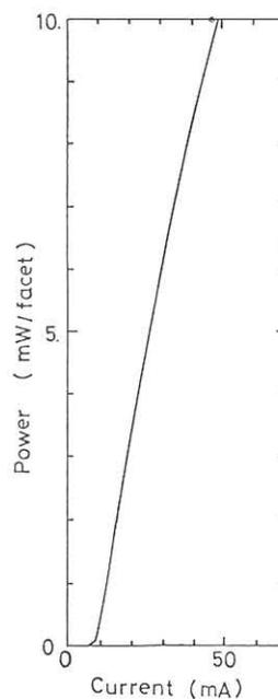
Fig. 4 The power-current characteristics of the low threshold current laser.
