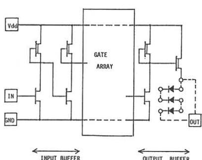
FIGURE.3 I/O buffer stages
